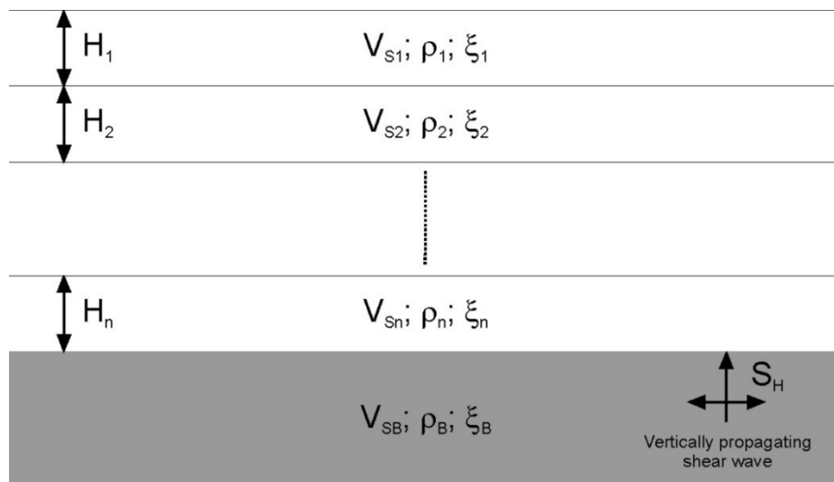
Fig. 2.1.1. One dimensional layered soil deposits system
