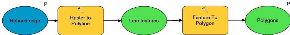
Fig. 2.9 - Flow chart of the Grain polygons creator routine. Legend as in Fig. 2.3.
