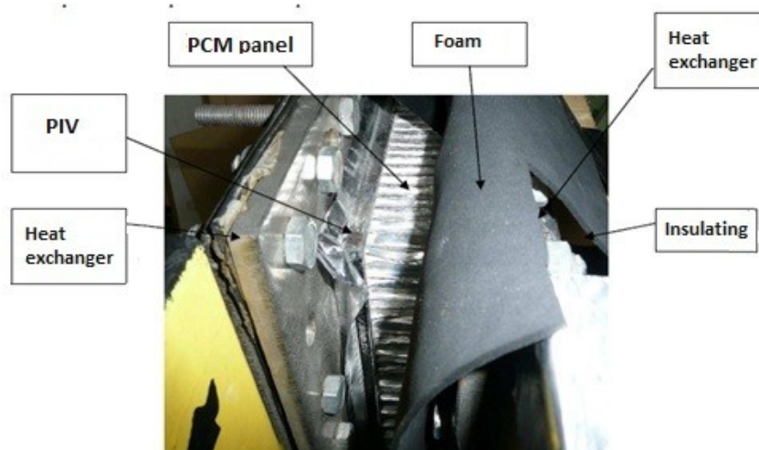
Fig. 15 Sample Panel tested by the CSTB.
