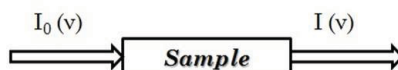
Figure 3.4: Pictorial representation of an absorption experiment; I_0 indicates the radiation incident on a sample, I the transmitted radiation and \nu its frequency [213].
