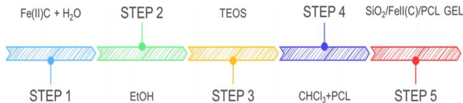
Figure 1. Flowchart of the sol-gel synthesis
