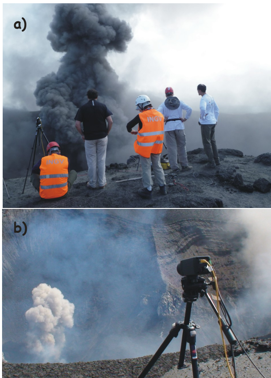
Figure 3.3: a) Experimental setup emplaced at Site1. b) Particular of the experimental setup: high speed camera filming explosions at Mt. Yasur. Photo courtesy of Piergiorgio Scarlato.
