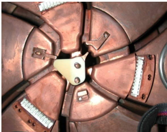
Figure 2.19: Central region of the CS. The housing surrounding the spiral inflector is also visible in the centre.
