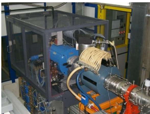
Figure 2.16: The CAESAR ion source at INFN-LNS.
