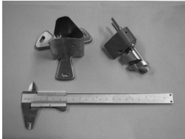
Figure 2.21: A picture of the housing and spiral inflector of the INFN-LNS Superconducting Cyclotron.
