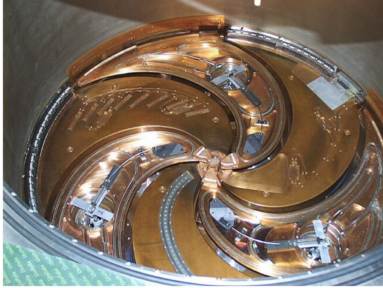
Figure 2.18: Accelerating structure of the CS. The phase slit system is also visible.
