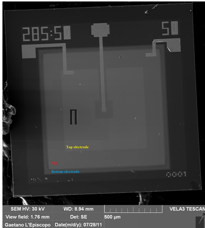
Fig. 2.18 – SEM picture illustrating the position of released cantilever beam inside the die previously used as ferroelectric capacitor. The areas occupied by the layers of the piezoelectric stack (top electrode, PZT and bottom electrode) are distinguished by the different shades of gray and indicated in the image for the sake of clearness.
