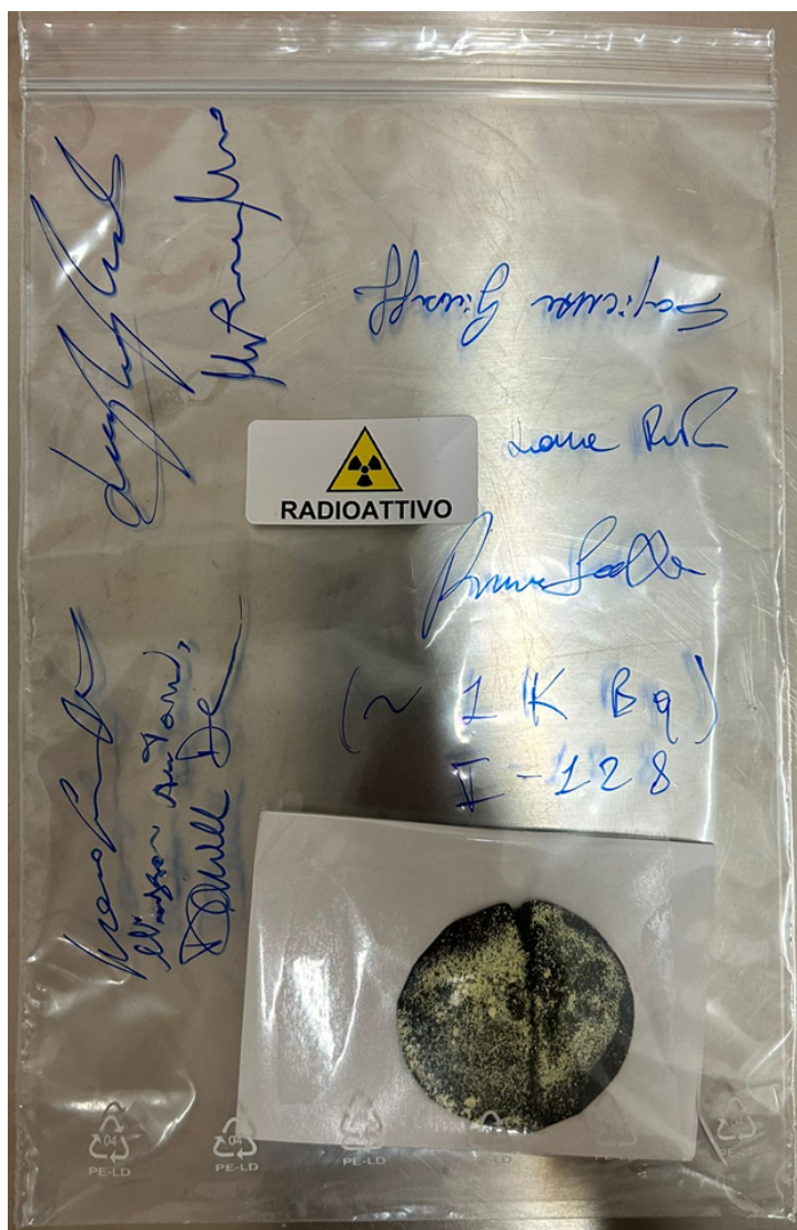
FIGURE 6.6: Radioiodine sample (in the form of yellow \text{Ag}^{128}\text{I} powder) as deposited on black filter paper at the end of the precipitation and of the whole extraction procedure.
