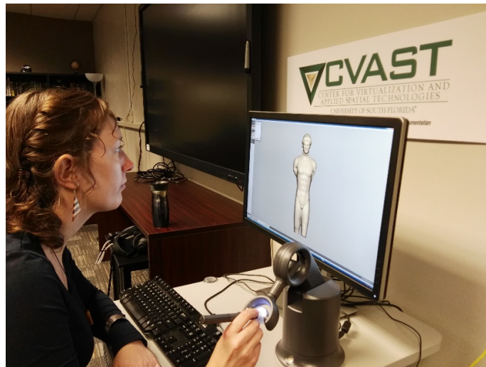
Figure A.44: Touch interaction with the digital model of the statue through haptic technology.
