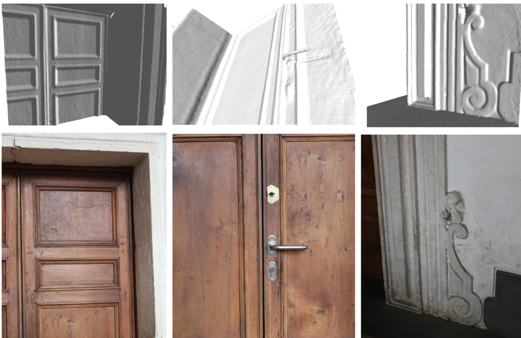
Figure A.30: View of the Structure Sensor behaviour on three different materials (from left to right): wood, metal, limestone.
