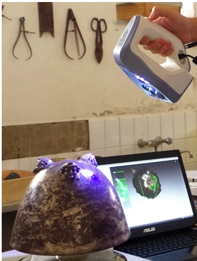
Figure A.12: Acquisition phases via 3D scanning of one piece of the collection.
