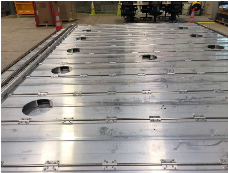
Figure 40. Photograph of one of the top cold shield panels after assembly.
