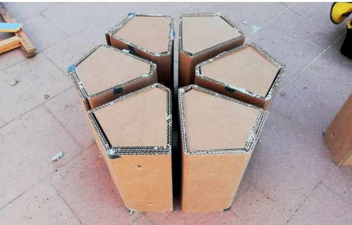
Figure 199 / Detail of tube-shaped corrugated cardboard profiles - On-site - University Campus, Catania (CT)
