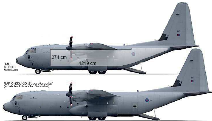
Figure 67 / ◀ CH-47 Chinook helicopter with container ISO 20, 2013 © U.S. army Capt. Peter Smedberg - via archive.defense.gov Figure 68 / ▶ C-130J Hercules II - © Ministero della Difesa - www.aeronautica.difesa.it Figure 69 / ▼ C-130J and C-130 J-30 size comparison
