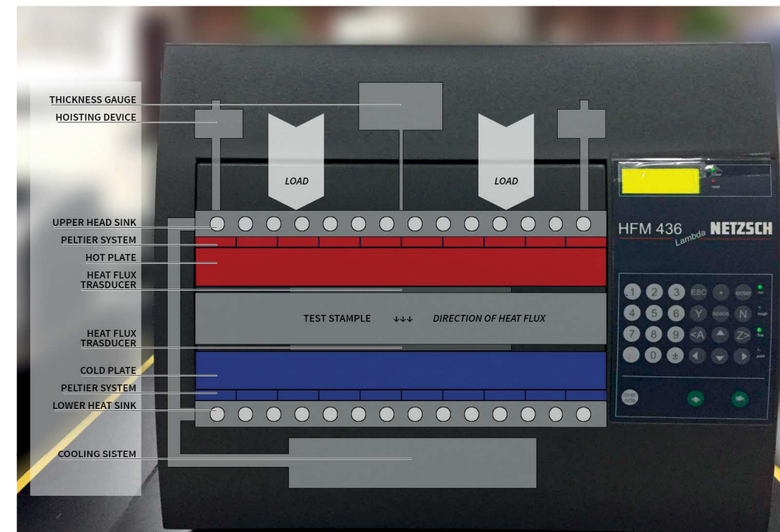
Figure 90 / Operating scheme of NETZSCH HFM 436 Lambda - © Dario Distefan
