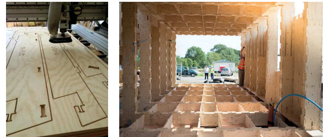
Figure 37 / ▼ Wikihouse CNC cutting and prototyping - © www.architecture00.net
