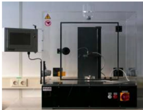
Figure 6:7 Electrospinning apparatus by IME Technology
