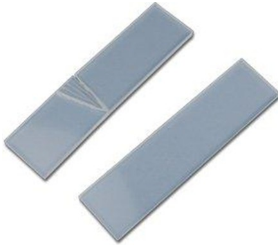
Figure 2:11 Damaged (top) and self-healed Veriflex EH epoxy
