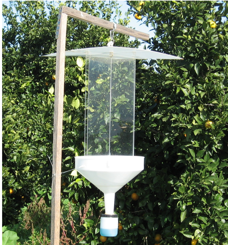
Fig. 3.1.1 – Active window trap in the sampling field (Photo A. Adorno).
