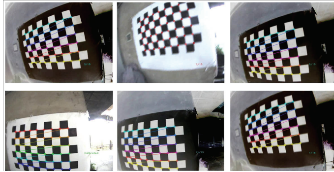
Figure 15 – A set of chessboard images used for the camera calibration process.
