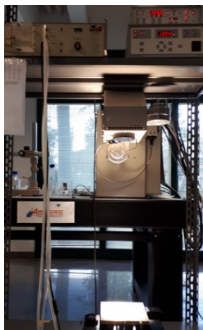
Fig. 3.3 – Overview of the CW solar simulator with its equipment, used for the tests indoor.
