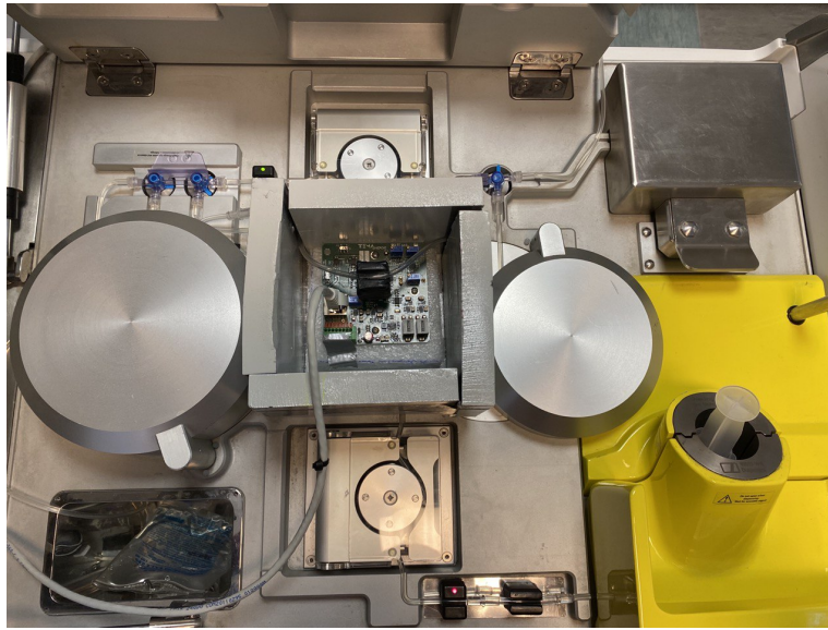
Figure 3.23: PVT detector placed on KARL100 dispenser inside a 2-cm shielding
