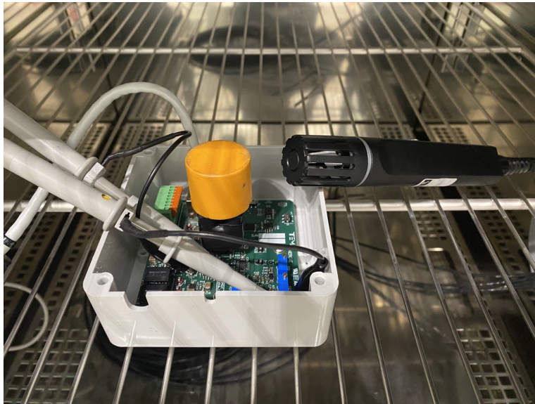
Figure 3.11: Source detector geometry inside climate chamber
