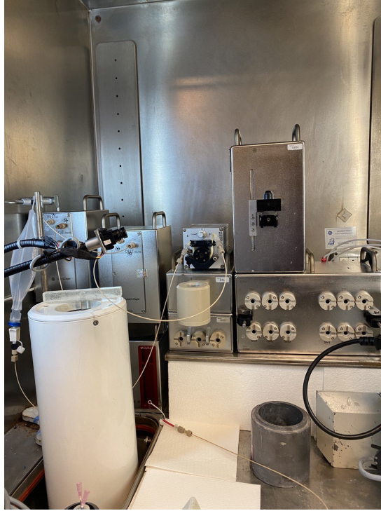
Figure 3.17: Three ^{68}\text{Ga} generators were connected in series
