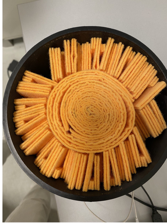
Figure 2.36: radioactive standard with gas density in Marinelli beaker geometry
