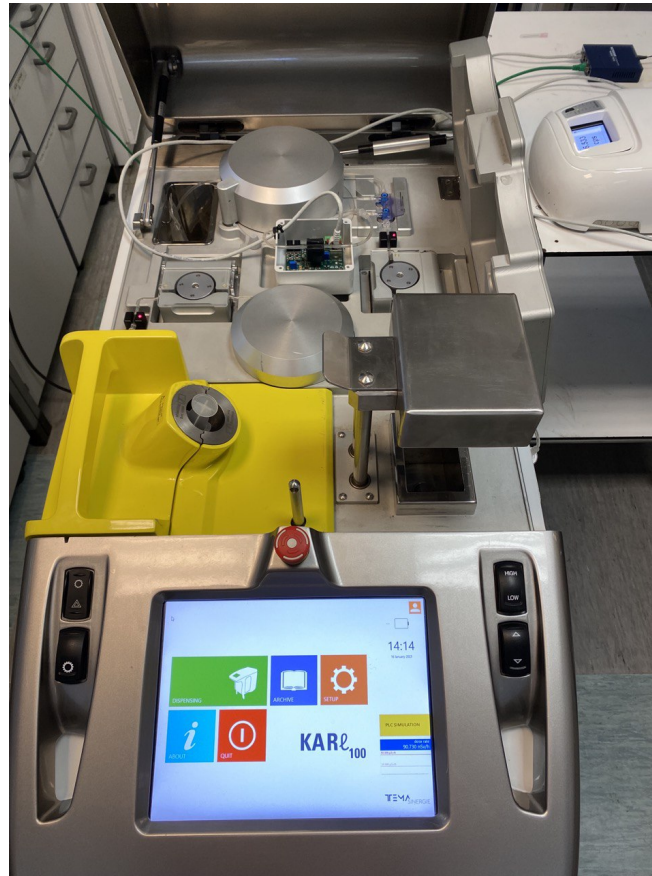
Figure 3.20: PVT detector placed on KARL100 dispenser
