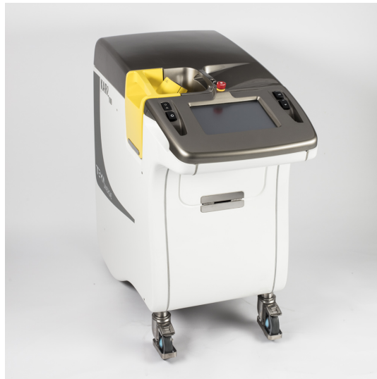
Figure 1.10: KARL100: An automatic dose dispenser in syringes made by Tema sinergie
