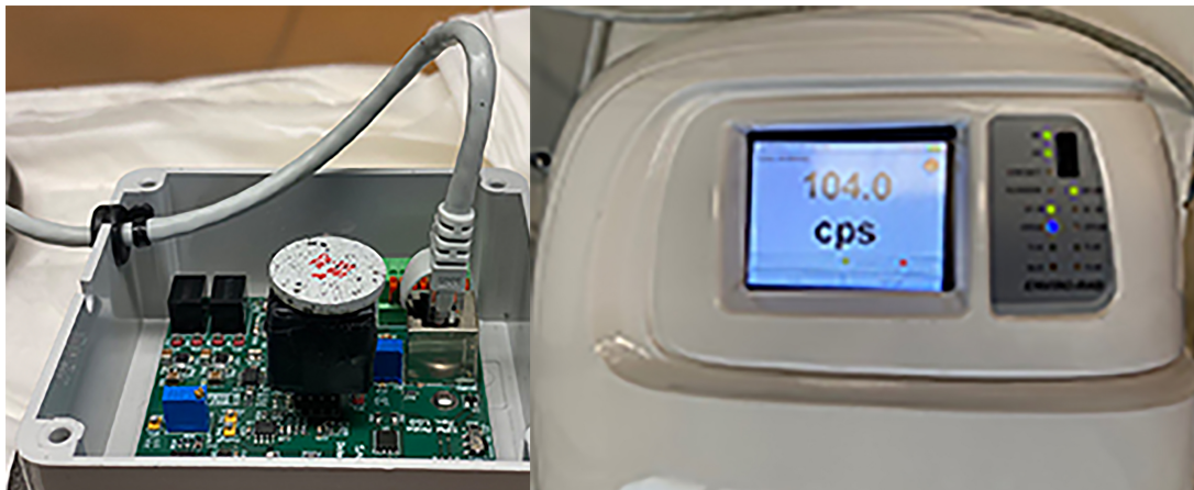
Figure 3.10: PVT detector system
