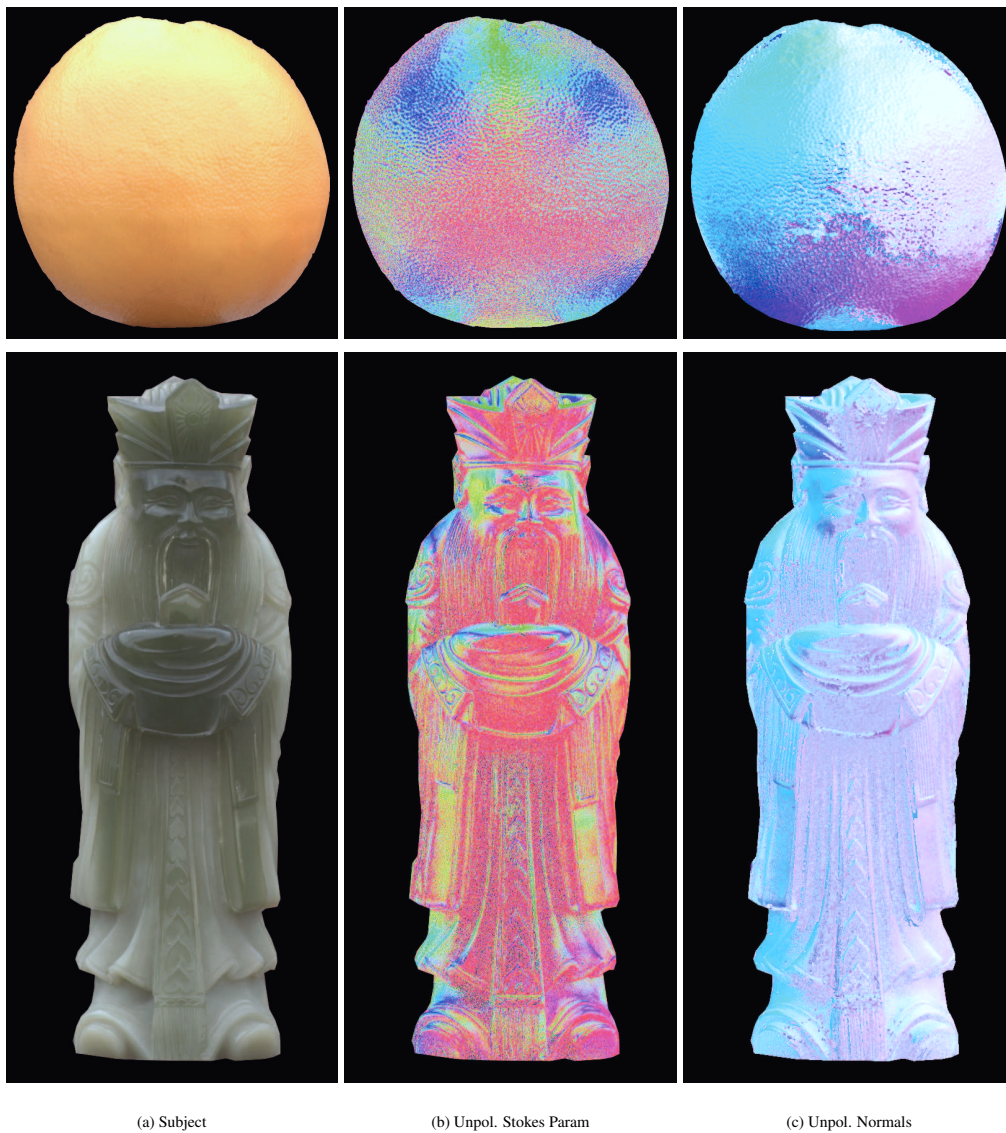
Figure 3.7: Estimated surface normals from Stokes parameters of diffuse outdoor illumination. Top-row: Plastic orange. Bottom-row: Confucius statue.
