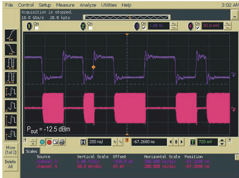
Fig. 3.23. Time-domain waveform of the transmitted signal (pink curve) and related data stream (violet curve).
