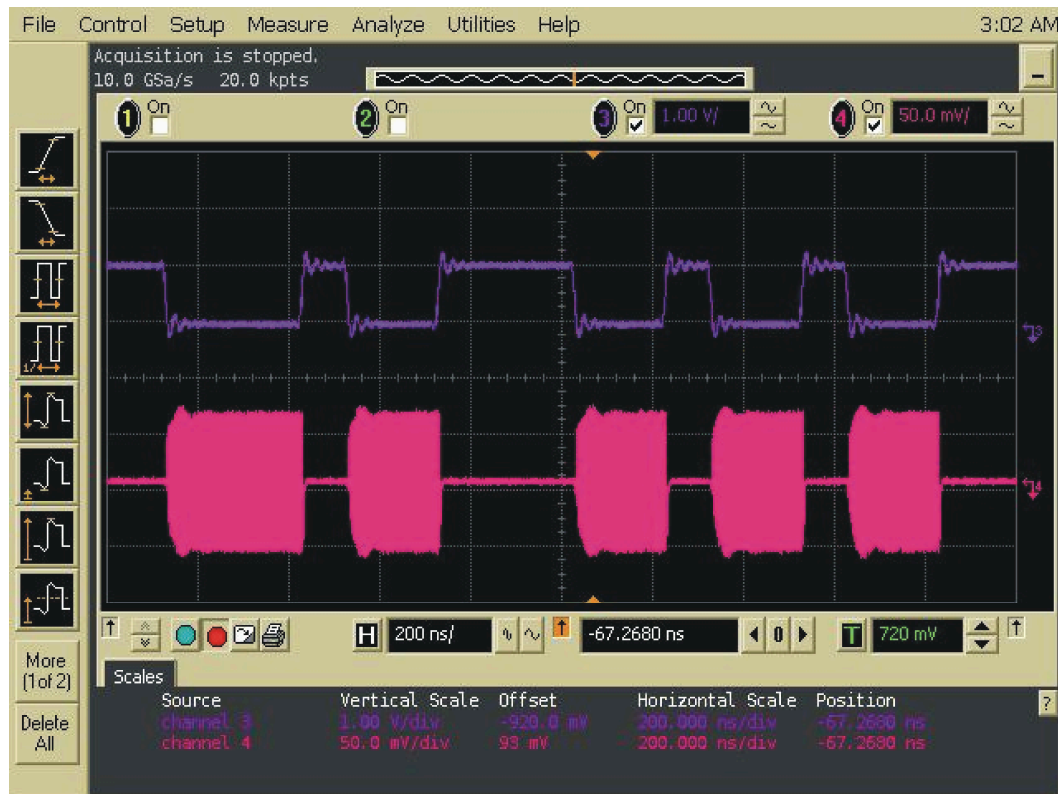
Fig. 3.32. Time-domain waveforms of the output data stream (violet curve) and the transmitted signal (pink curve).
