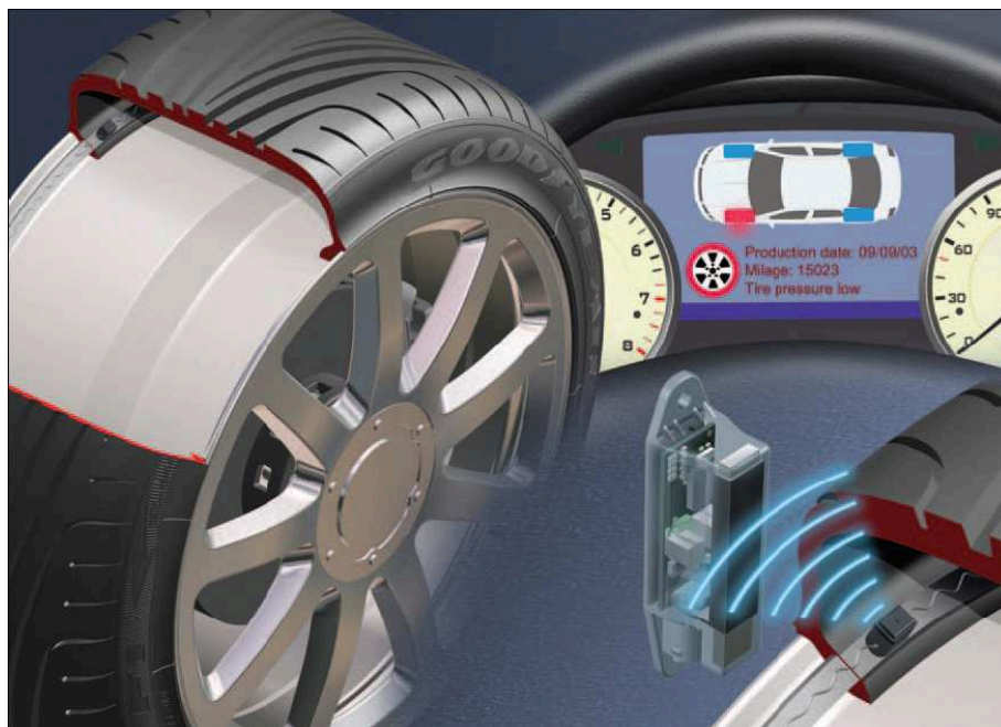
Fig. 1.2. Tire pressure monitoring system.
