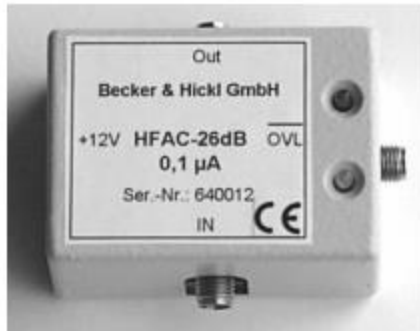
Figure 5.9: Becker & Hill HFAC preamplifier. Main characteristics of this device: 26 dB amplification with cutoff frequency of 1.6 GHz [84]
