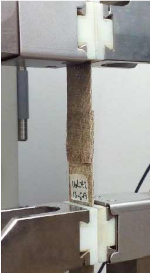
Fig. 5.20 | Provetta di SEBS-Biotex sottoposta a Single-lap joint shear test
