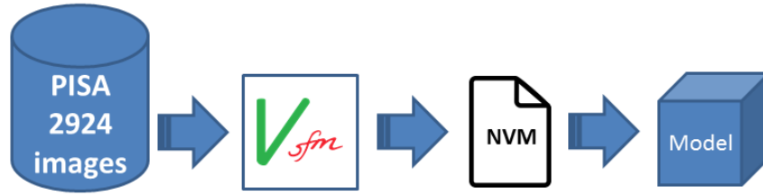
Figure 3.1: VSFM integration initial workflow: images of a collection are processed with VSFM and a Model is obtained through parsing of the NVM file and aggregation from our framework of meta-data.
