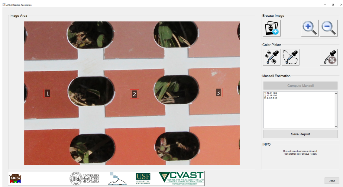
Figure A.3: Screenshot of the ARCA desktop application GUI. Three samples have been taken on the current image; marks are visible on the image so the user can visually track the estimated Munsell values. Now the user can keep sampling the image (adding new Munsell estimations) or save a report of the current estimation.
