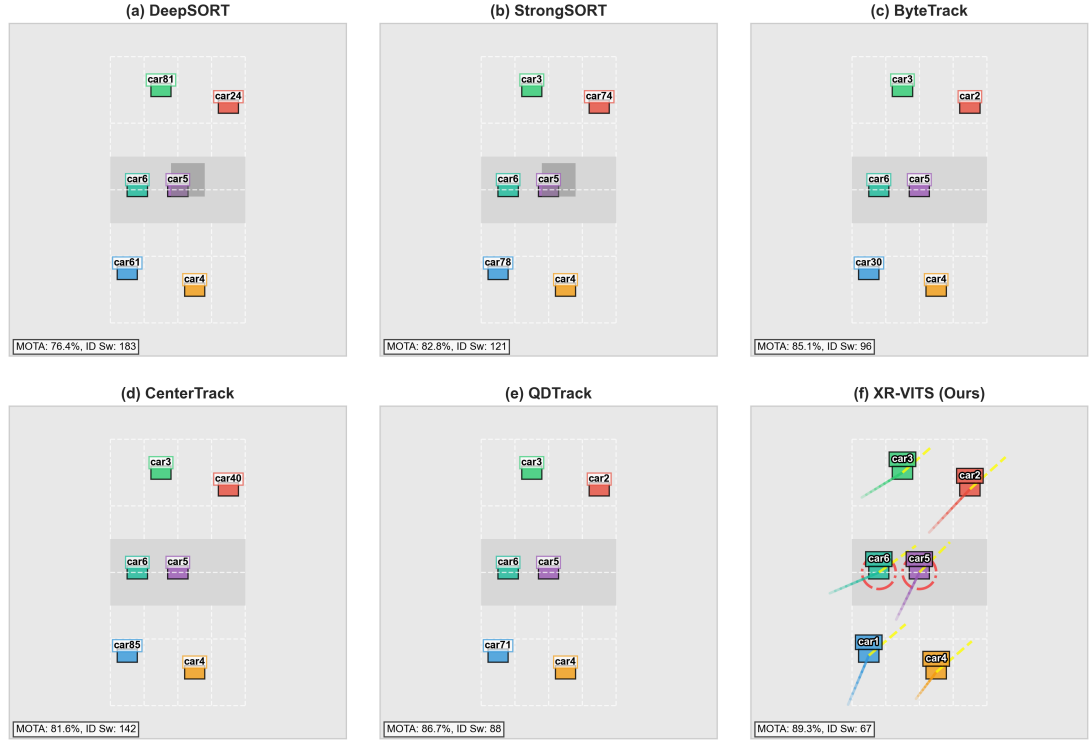
Figure 5.3: Visual comparison of tracking performance. (a) DeepSORT, (b) StrongSORT, (c) ByteTrack, (d) CenterTrack, (e) QDTrack, (f) XR-VITS (Ours). Note how XR-VITS maintains ID consistency through occlusions at the intersection.
