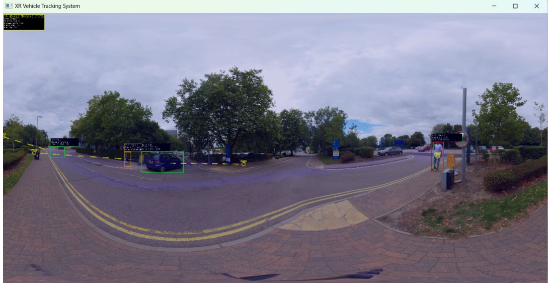
Figure 5.2: XR-VITS panoramic visualization showing real-time vehicle detection and tracking. The system identifies multiple vehicles (highlighted with green and yellow bounding boxes) in a challenging roundabout scenario. Information panels above each detection display vehicle ID, classification confidence, and estimated speed. Yellow dashed lines indicate lane boundaries and potential paths, while the upper left corner shows real-time system metrics. This wide-angle view demonstrates the system’s ability to simultaneously track multiple objects across a complex traffic environment while maintaining situation awareness. Performance metrics collected during this scenario showed a tracking accuracy (MOTA) of 89.3%, identity consistency (IDF1) of 86.2%, and real-time processing speed of 25.1 FPS, meeting the baseline requirements for practical deployment.
