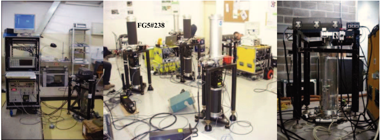
Figure 2.4 – International and European Absolute Comparisons: on the left the IMGC-02 during the ICAG 2005; in the middle the FG5#238 during the ICAG 2009; on the right the IMGC-02 during the ECAG 2011.
