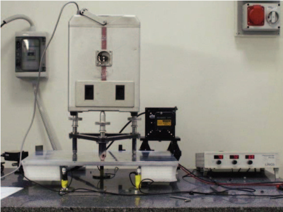
Figure 4.6 – Experimental set-up used for the determination of the coupling degree between high-frequency vertical accelerations and the In-band response of the Scintrex CG-3M. The figure shows the piezoelectric actuators placed below the movable platform.
