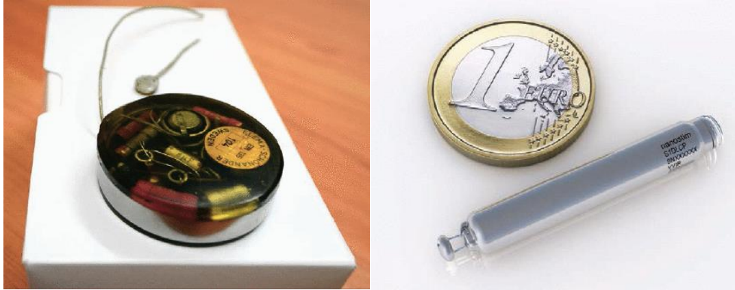
Figure 1.10: Picture of the first pacemaker implanted in USA 1960, the electrode has two small holes to be sutured to the epicardium (left) and Current development to 'The Nanostim leadless pacemaker' which is less than a 10% of the size of a conventional pacemaker (right) [40]
