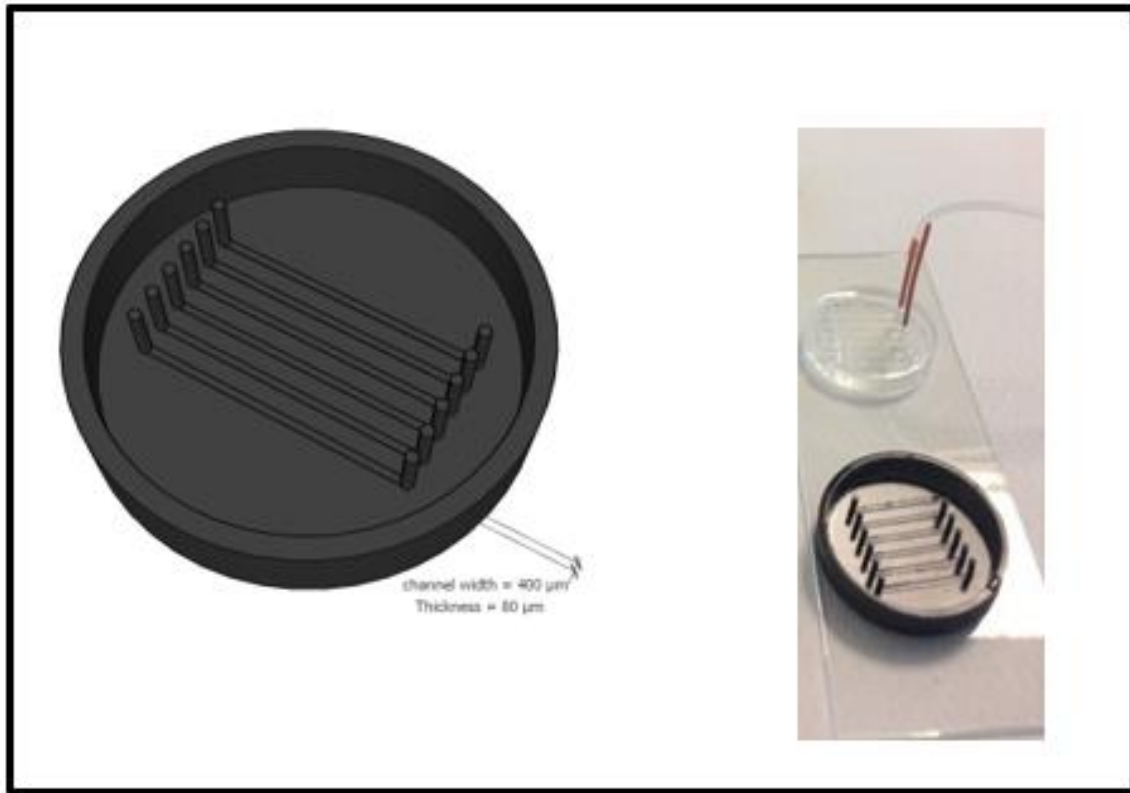
Figure 4.15: Master geometry after design with 3D cad software SketchUP®. Snapshot of the 3D printed master(Left) and a PDMS replica with PEEK tubings for connection with external(Right)
