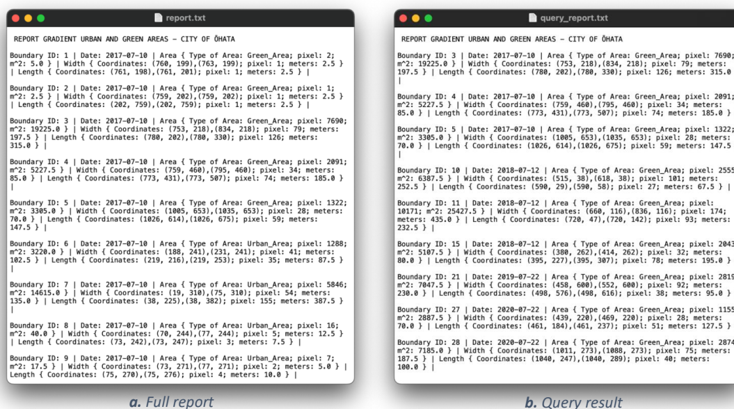
Figure 4.8: Two types of reports are obtained at the end of processing: (a) a complete report which contains the data of all the new boundaries identified in the image; (b) report showing data filtered by a query based on certain conditions (green areas with surfaces greater than 1000 pixels).
