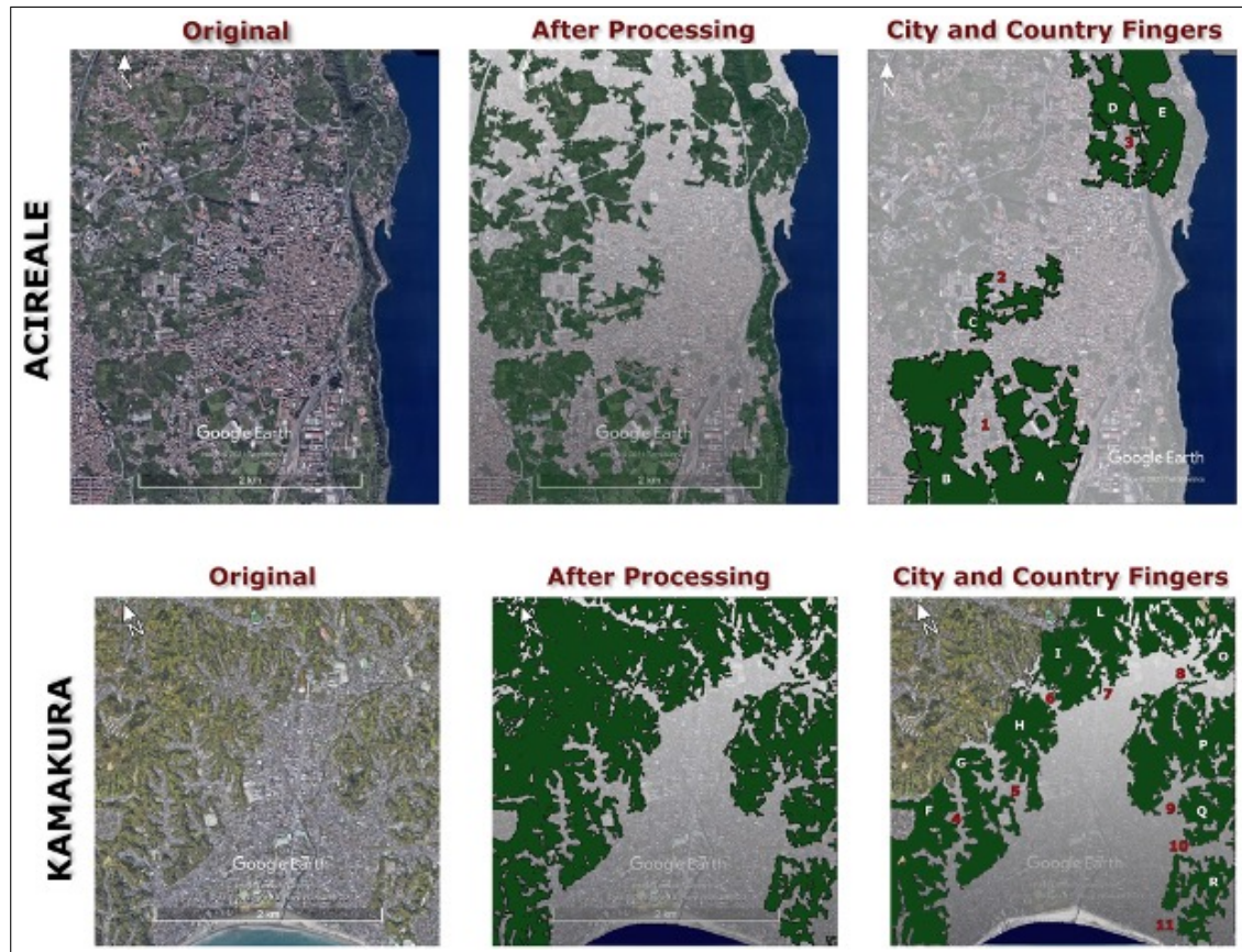
Figure 3.5: The results of the image processing of the Acireale and Kamakura cities. In the figures on the left the original image, in the central ones the result after the processing phase and in the figures on the right of the country and city fingers for both places indicated by letters and numbers. The vegetation is shown in green and the urban center in transparent gray
