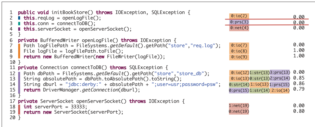
Figure 4.6: Apply extract method refactoring to separate clustered concern tags and enhance concern cohesion.
