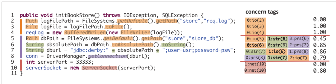
Figure 4.5: Concern tags given by the proposed approach can be used to suggest refactoring opportunities. Using a clustering algorithm, three blocks of source lines having similar concern tags have been found (i.e. three different clusters ): line 2 to line 4 ( C0 , indicated by the orange vertical line); line 5 to line 8 ( C1 , indicated by the purple vertical line); and line 9 to line 10 ( C2 , indicated by the red vertical line). The identified clusters actually refer to the three different subtask performed by the method: open the log file, open the database connection, and open the server socket, thus automatically suggesting a method decomposition into smaller and concern cohesive methods.
