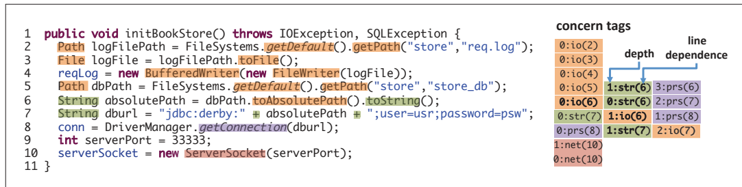
Figure 4.4: The second step of the concern tagging approach. By using a taint analysis approach, all the concern tags given by the previous step (i.e. directly accessing a Java API, thus having a ‘0’ depth value) are now used as sources for a concern related data flow that we can trace to discover all the instructions implicitly sharing the same concern of the source. All the concern tags having a depth value greater than ‘0’ have been discovered using this taint analysis propagation. For example, let us consider the concern tags generated by line 6 (highlighted by the use of bold text): the io and str tags have been backward propagated to line 5 due to the data dependence made by the dbPath variable, and forward propagated to line 7 and line 8 in turn due to the absolutePath and the dburl dependence.
