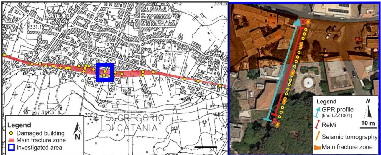
Fig. 6.5. The box at left shows the location of the investigated area; the box at right shows the location of G.P.R., ReMi and seismic tomographic surveys (modified after Imposa et al., 2015a).
