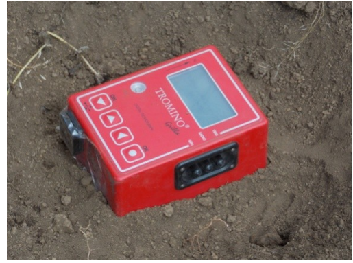
Fig. 6.13. Three-components seismographs (Tromino)
