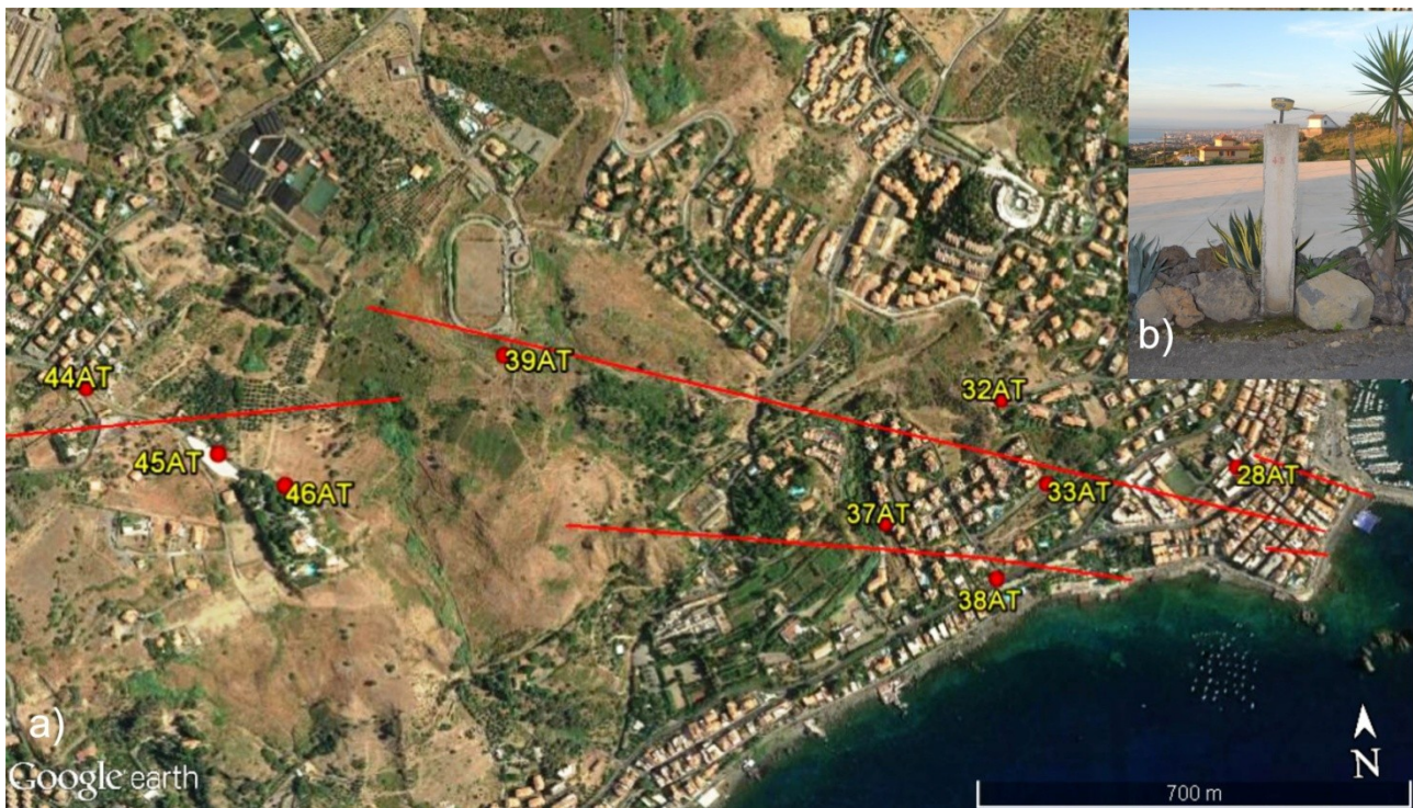
Fig. 6.52. a) Geodetic monitoring network of ATF fault segments; b) photograph of a monitoring point (45AT)
