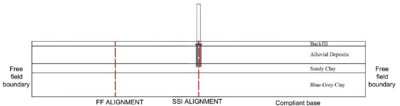
Figure 19. Vertical alignments: along the structure (SSI) and far from the structure (FF).
