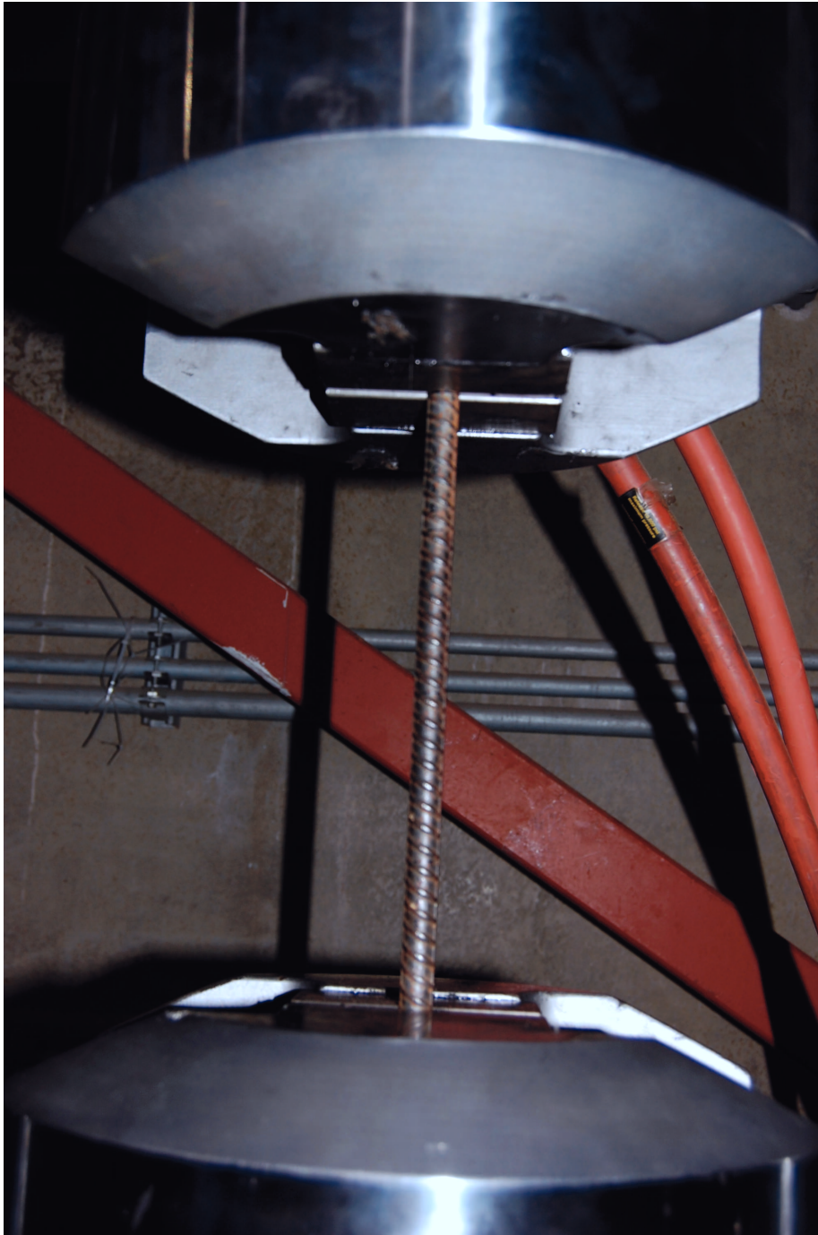
Figure 3.13: A706 steel test sample, 9 db
