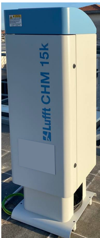
Figure 3.1: EHT's Lufft CHM 15k lidar-based ceilometer.
