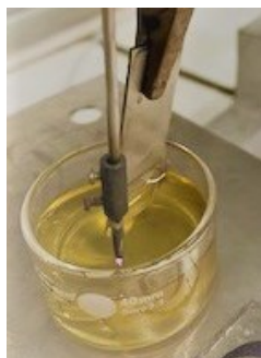
Figure 5.1. Synthesis of the HA@Ag(P) and the experimental apparatus ( \text{AgNO}_3 1mM, HA 0.2 mg mL -1 ).
