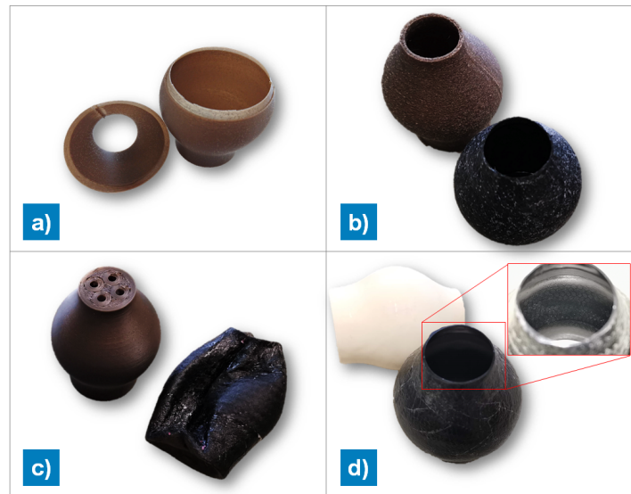
Figure 3.7: AM mandrels: a) FDM - shell 1 mm, b) FDM - shell 2 mm c) FDM - collapsed sparse design after applying the autoclave pressure (5 bar), d) LCD - breakable 2 mm mandrel with particular on the good internal surface quality.
