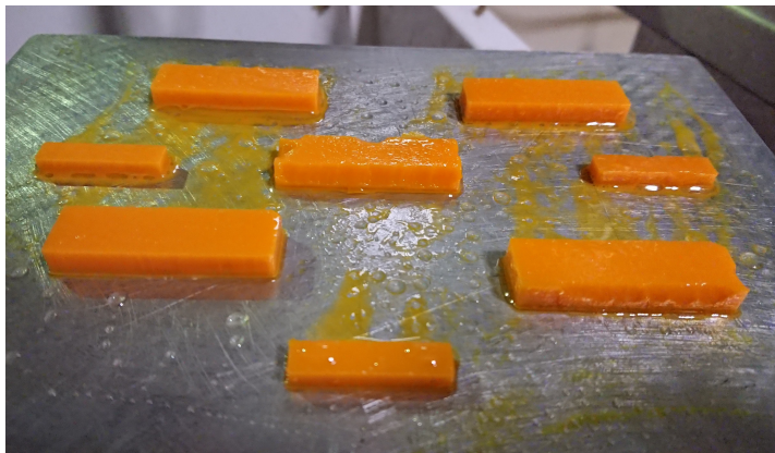
Figure 3.18: Printing trials for the CE7030 blend with the optimized printing conditions after photocuring optimization (see Table 3.4).
