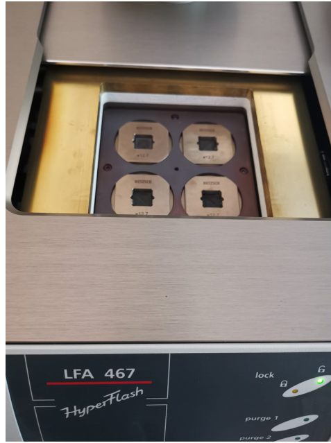
Figure 2.9: Laser Flash test setup.
