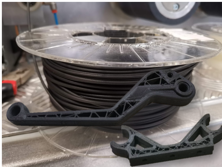
Figure 2.8: 3D printing components by PLA+CF30.
