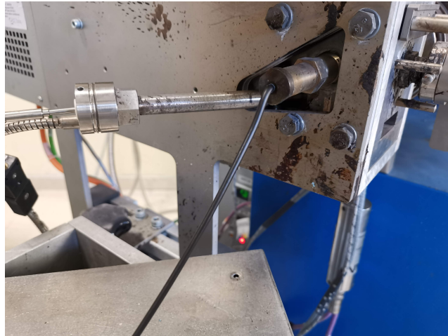
Figure 2.2: Particular of PLA CF-reinforced filament extrusion.
