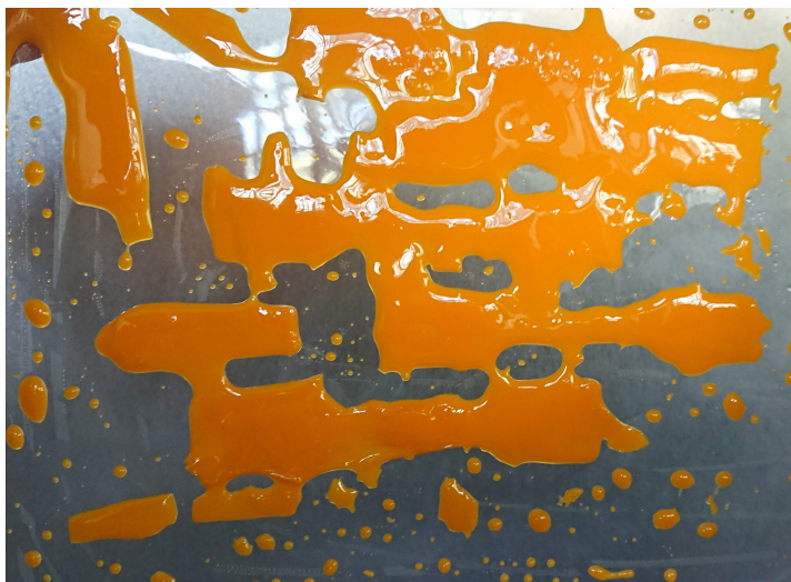
Figure 3.17: Printing trials for the CE7030 blend with the same printing conditions used for the cream resin (see Table 3.4).
