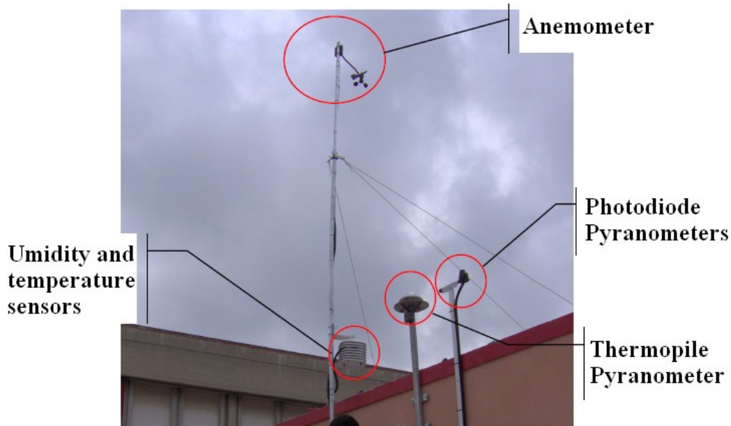
Figure 4.9: Weather Station WSENSmeteo (the anemometer is placed at the top of a 4 m high pole).
