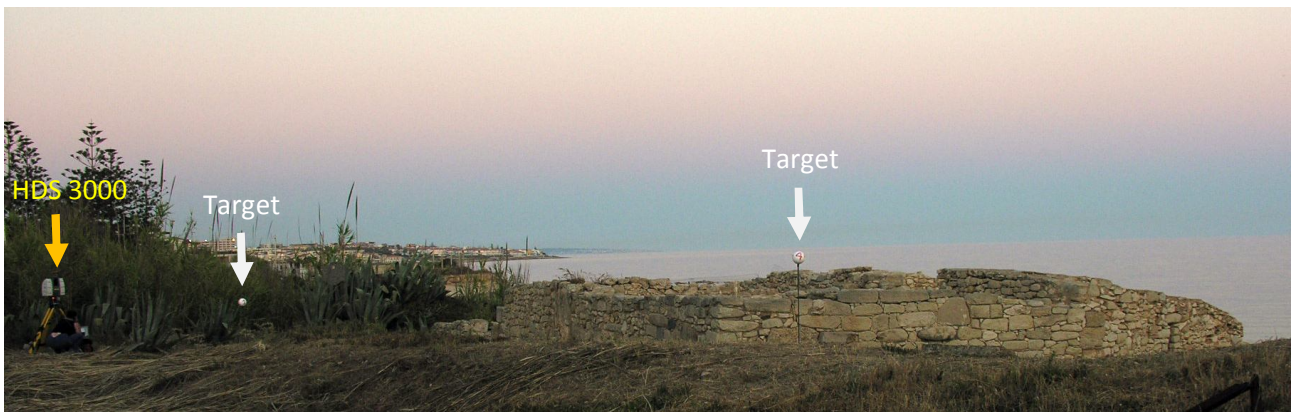
Fig. 10: Experimentation on the field with 3D spherical target.
