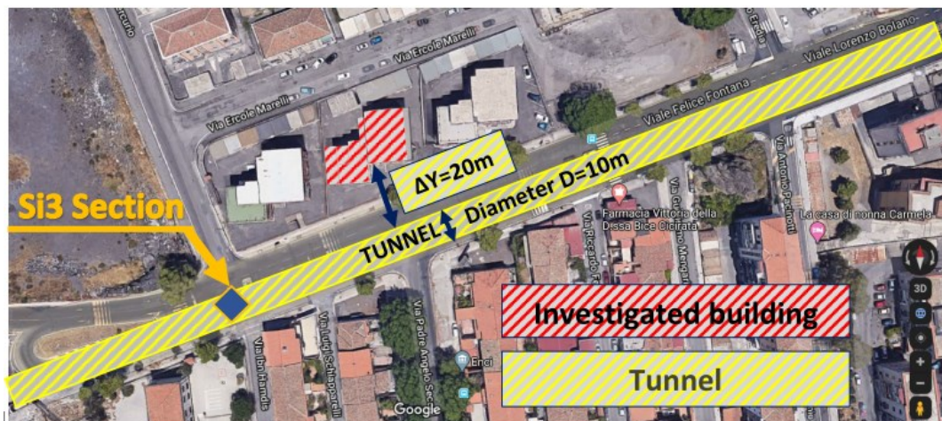
Figure 4.31: Position of the building and the tunnel modelled by means ADINA code
