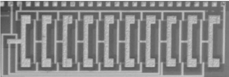
Fig. 2.30. Photograph of the 7-stage CMOS ring oscillator.
