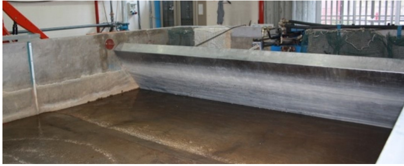
FIGURE 6.2 Paddle of the flap-type wave-maker of the wave tank of the Hydraulic Laboratory of the University of Catania.
