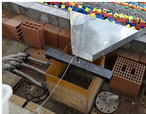
FIGURE 6.9 System for the measurement of the mean overtopping discharge per meter ( q ) placed behind the physical model.
