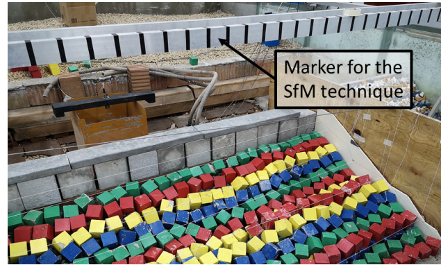
FIGURE 6.7 Marker used to scale the 3D point clouds of the model recovered by means of the SfM technique.
