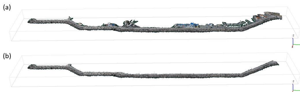
FIGURE 4.3 Point cloud of the Catania harbor breakwater produced from UAV survey of February 2020 (coordinate system WGS84/UTM zone 33N, EPSG: 32633, resolution equal to 1940 points/m 2 ): a) whole point cloud (299,677,460 points); b) point cloud of the region of interest (192,557,211 points).
