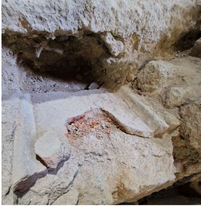
Figure A.6: Sampling point of the Rot_C_M12 mortar, collected from the inner portion of one of the hydraulic ducts in area C. The sampling was performed by removing the inner mortar core to minimise light exposure and surface contamination.
