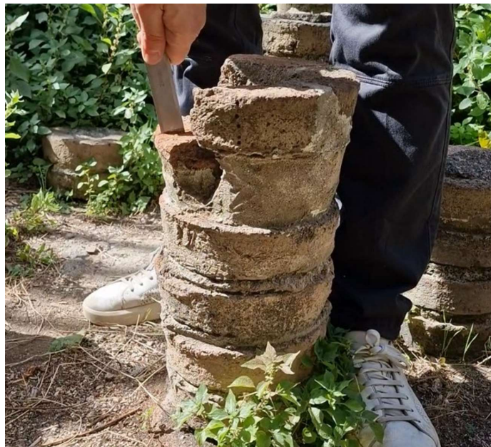
Figure A.21: Sampling point of the Rot_D_M3 mortar, collected from the inner portion of a pila (brick column) located in the hypocaust system of the hot room at the Terme della Rotonda. The inner core of the mortar was extracted to minimise exposure to light and surface contamination.
