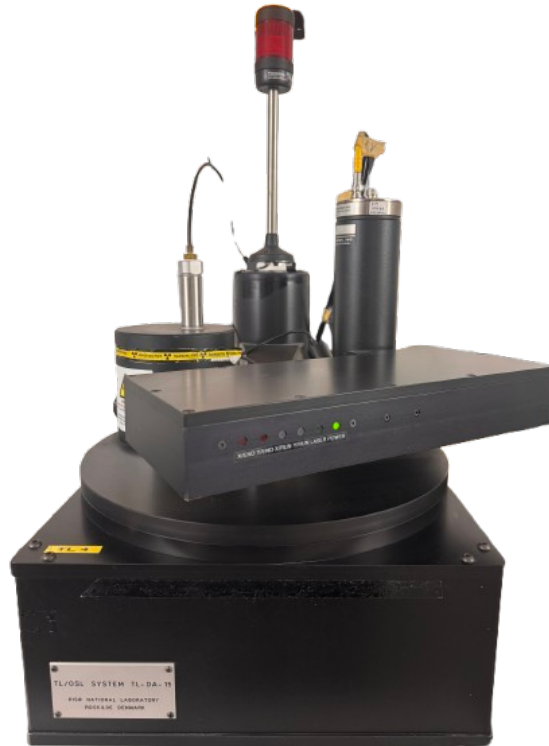
Figure 3.4: Automated luminescence reader used in this study: Risø TL/OSL DA-15.
