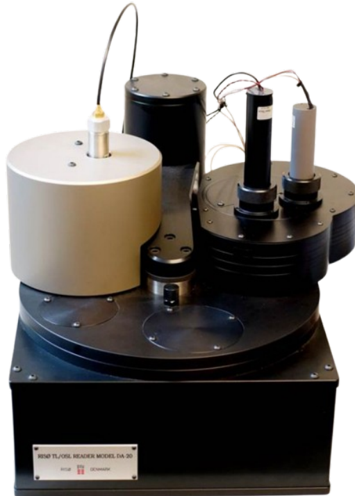
Figure 4.4: Risø TL/OSL DA-20 reader employed for SG-OSL measurements in this study.
