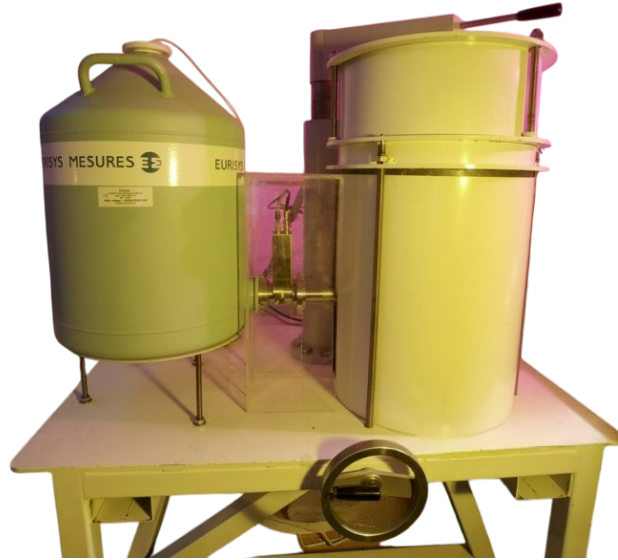
Figure 4.17: HPGe gamma spectrometry detector (EGPC 200 P17, Canberra-Eurisys). Adapted from [131].
