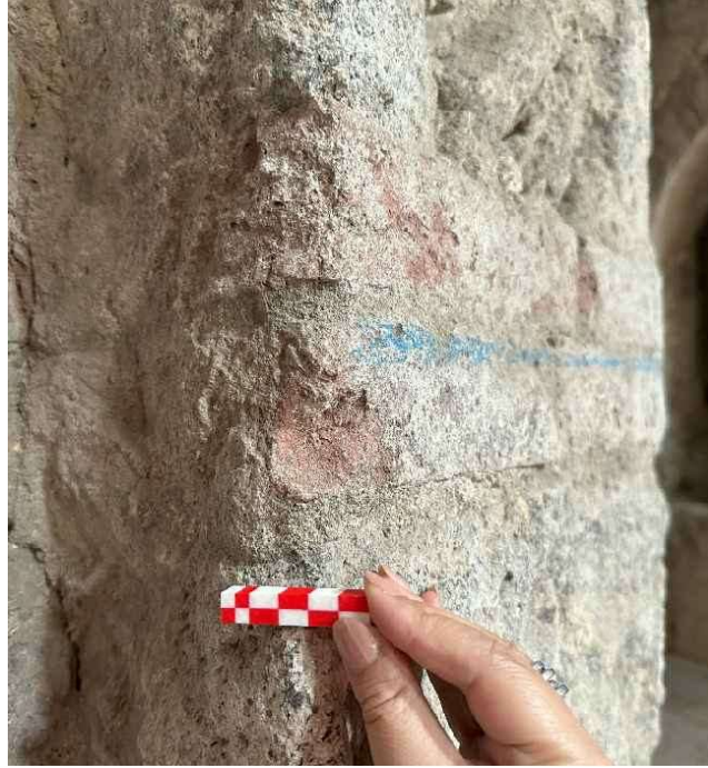
Figure A.11: Sampling point of the Rot_C_M14 mortar, extracted from the inner section of a wall in area C. The preserved underlying mortar was accessed to minimise light exposure and avoid surface contaminations.
