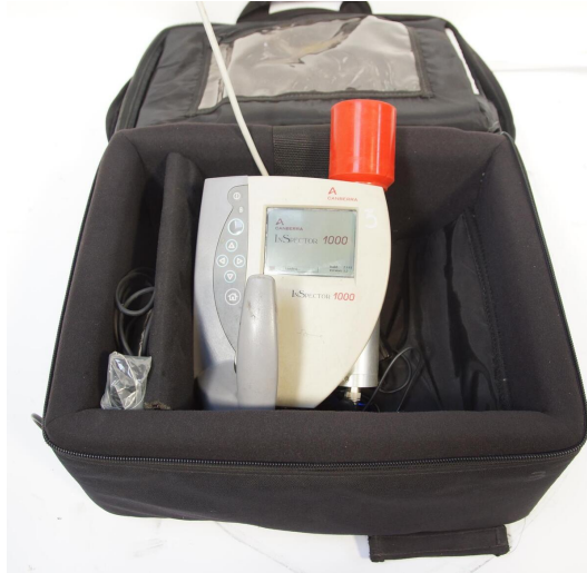
Figure 4.18: Portable gamma spectrometer (Canberra Inspector 1000) used for in situ dose rate measurements.
