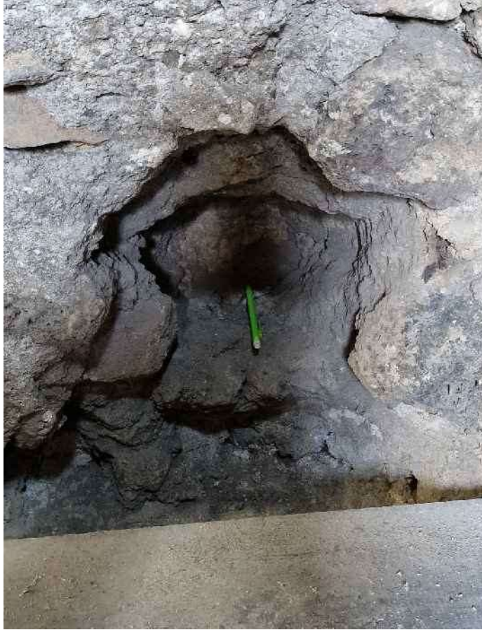
Figure A.1: Sampling point of the Rot_C_M11 mortar, collected from the inner portion of a wall in area C, corresponding to the frigidarium of the Terme della Rotonda. The inner core of the mortar was extracted to minimise light exposure and surface contamination.
