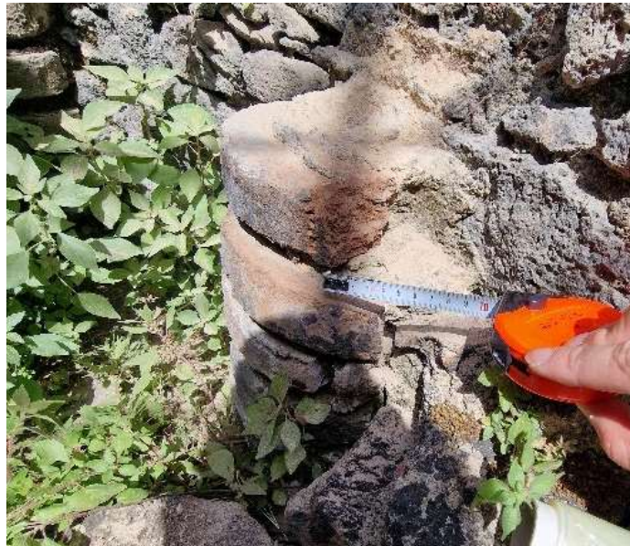
Figure A.26: Sampling point of the Rot_D_M5 mortar, collected from the inner portion of a pila . The inner core of the mortar was extracted to minimise exposure to light and surface contamination.
