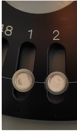
Figure 3.5: Stainless steel cups mounted in the Risø carousel, each containing a monolayer of sample grains fixed with silicone spray. These holders were used for multigrain TL measurements in this study.
