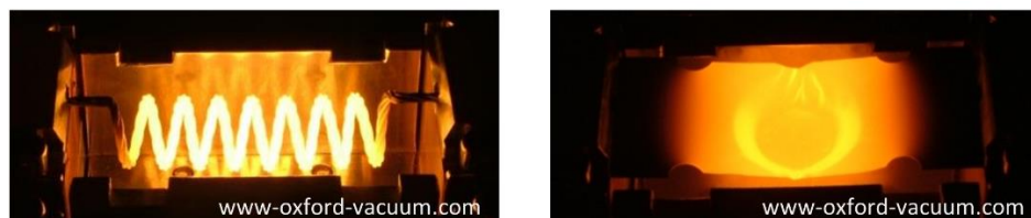
Figure 2.4. Examples of resistive elements for thermal evaporation: spiral tungsten filament (left); dimpled boat in a resistive media (right).
