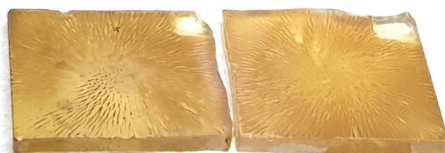
Figure 4.4. Striation defects in perovskite precursor films obtained by adding 25 g/L of \alpha -terpineol to the precursor solution.
