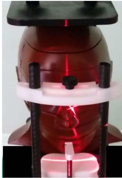
Figure 1. Head–neck phantom positioned in the cone beam computed tomography (CBCT).
