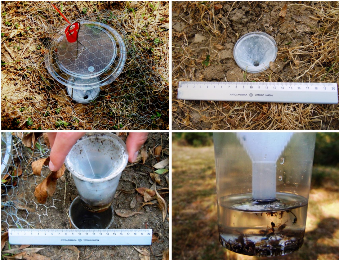
FIGURE 11 – TRAPS IN THE GROUND. It is often advantageous to use an obvious marker for each trap, such as a flag, to aid in relocation. (Photos © LI VIGNI, 2011)
