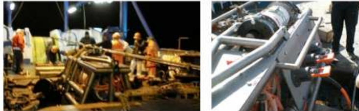
Figure 4.2: The Capo Passero deep-sea Junction Box, successfully deployed in November 2009. A detail showing the three ROV operable connectors is shown on the right.
