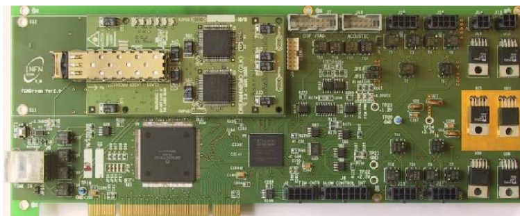
Figure 4.13: Picture of the Floor Control Module Board (FCMB).
