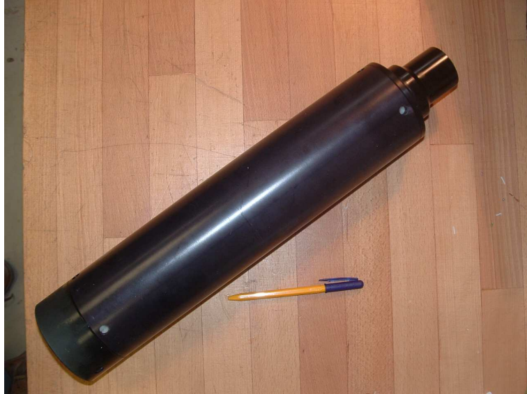
Figure 5.13: Picture of an ACSA beacon used for the positioning of the NEMO-SMO detector.
