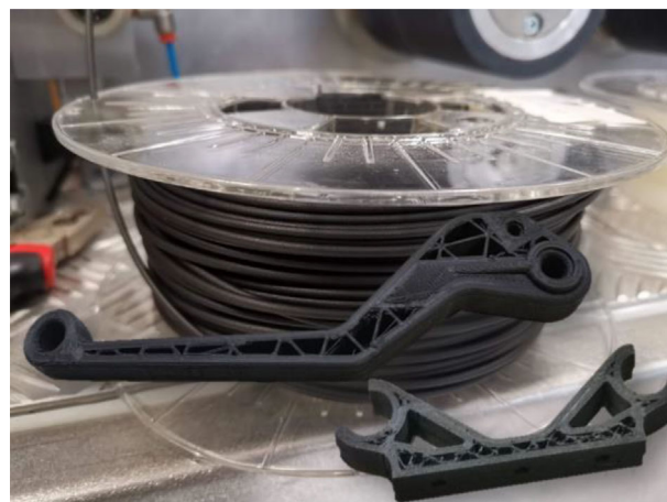
Figure 5. 3D printing components by PLA+CF30.
