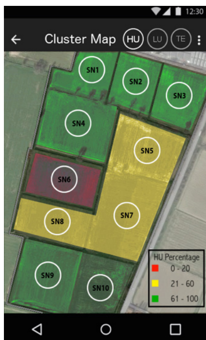
Figure 14 - Application prototype to manage agricultural lands: the field is divided into clusters grouped by soil moisture value
