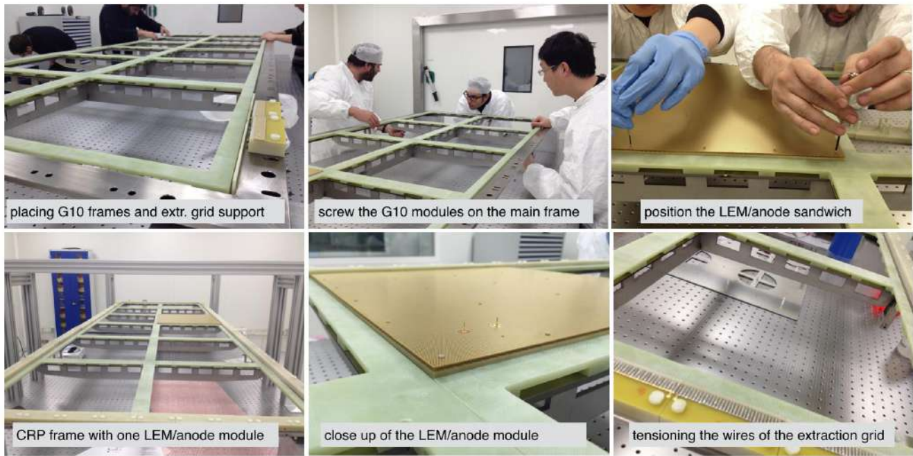
Figure 5.16: Pictures of the assembly of a 3 \times 1\text{m}^2 CRP
