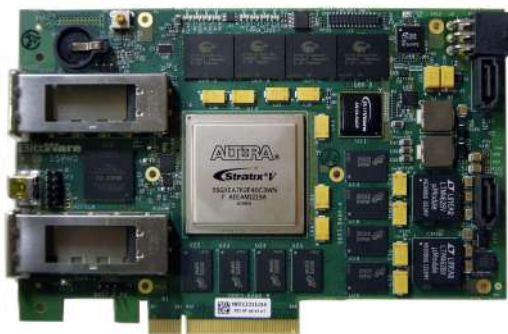
Figure 5.25: FPGA processing board based on Stratix V from Altera. The board features a dual QSFPP+ cages for 40GigE or 10GigE links, 16 GBytes DDR3 SDRAM, 72 MBytes QDRII/II+, two SATA connectors and is programmable via OpenCL.
