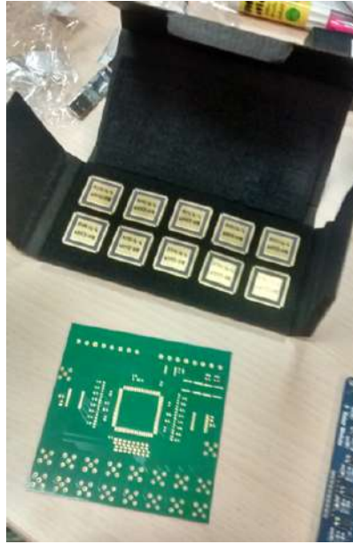
Figure 5.19: Front-end 16 channels cryogenic ASIC amplifier with the double-slope gain implementation
