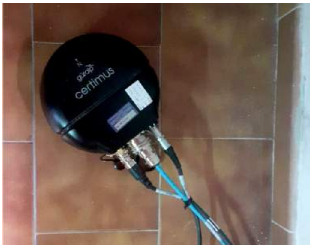
Figure 4. Guralp Certimus digital seismic sensor during a laboratory test.
