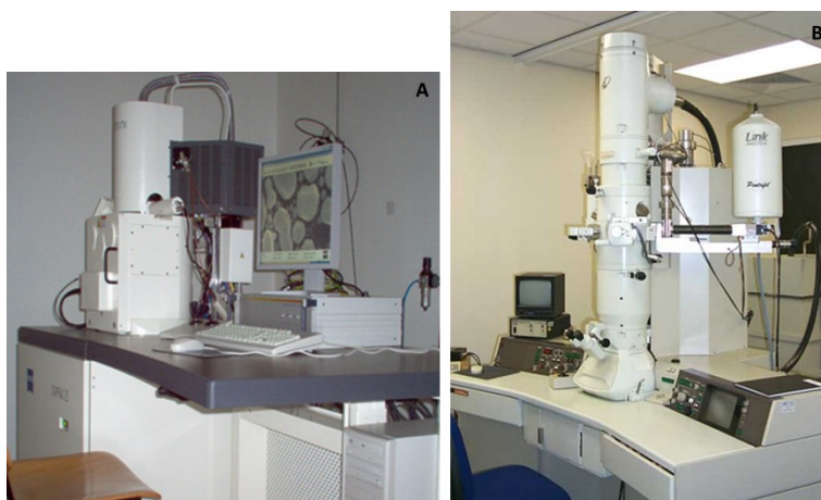
Figs. 16. A) Scanning Electron Microscope (SEM) Zeiss Supra 25; B) Transmission Electron Microscope (TEM) Jeol JEM-2010F.
