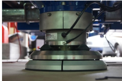
Figure 8 - Loading plate of 300 mm. FWD Dynatest 8000 (University of Catania)
