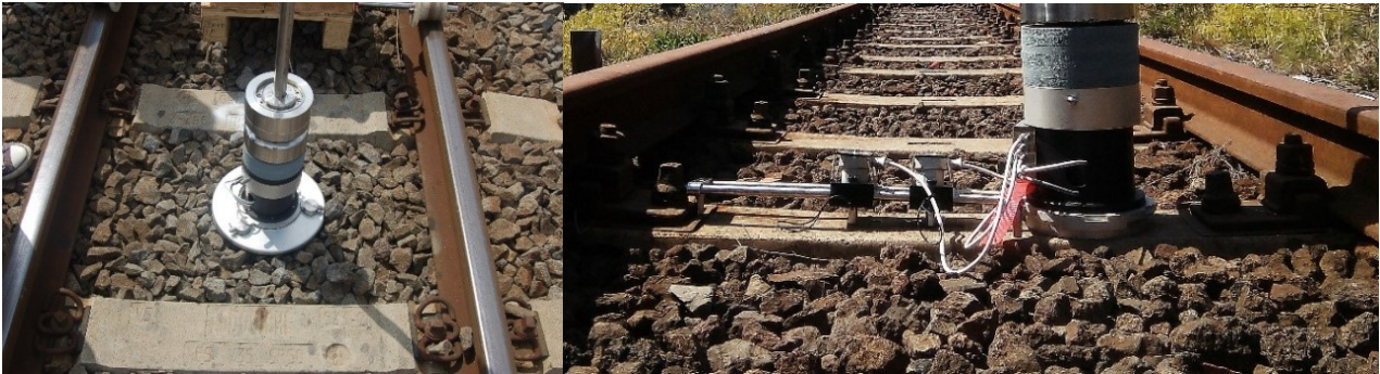
Figure 33 - LWD test with plate in crib position and with plate on the sleeper with additional geophones
