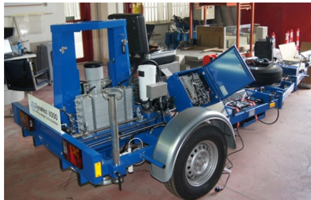
Figure 7 - Falling Weight Deflectometer 8000 (University of Catania)
