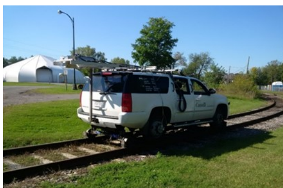
Figure 30 - Multifunctional vehicles used by Pavemetrics to test the LCMS performance on surveying railway tracks
