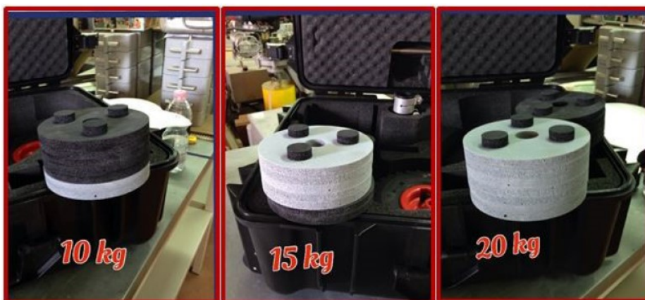
Figure 15 - Buffer configurations at 10 - 15 - 20 kg. Dynatest LWD 3031, University of Catania
