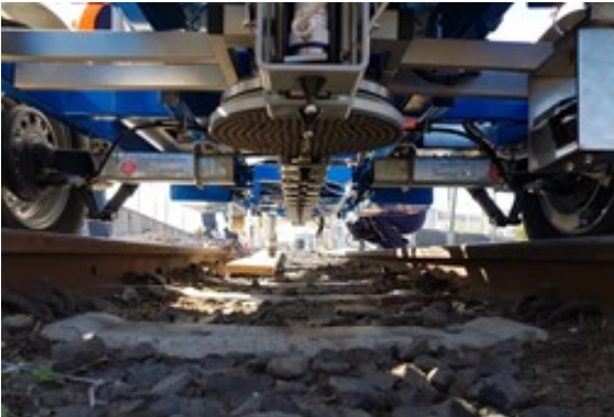
Figure 34 - FWD test position
