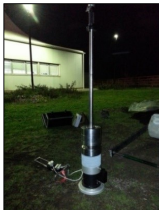
Figure 59 - Light Weight Deflectometer in the area test of the University of Catania
