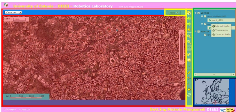
Figure 89 – WebGIS components: legend area (green), map area (red), reference map (blue) and toolbar (yellow)
